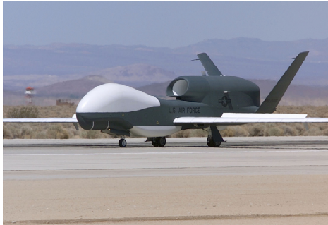
Figure 3. Global Hawk and Predator are examples of unmanned aircraft that went into limited operation before being certified by conventional structural test methods.
